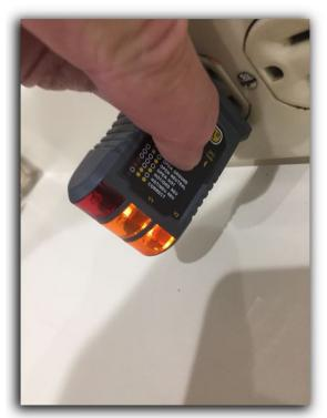
21. <u>Not all of the kitchen counter top receptacles appear to be connected to a ground fault circuit interrupter (GFCI) device.</u> When a GFCI tester was engaged, the circuit remained live. Under current electrical standards, all kitchen counter top receptacles should have GFCI protection. Recommend further
